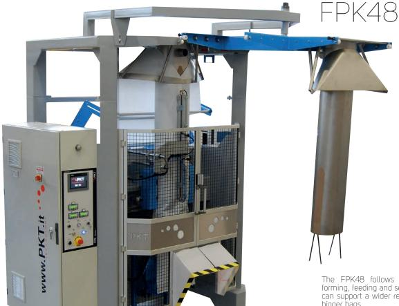
The FPK48 follows our FPK64 in the forming, feeding and sealing components. It can support a wider reel widths to produce bigger bags.
